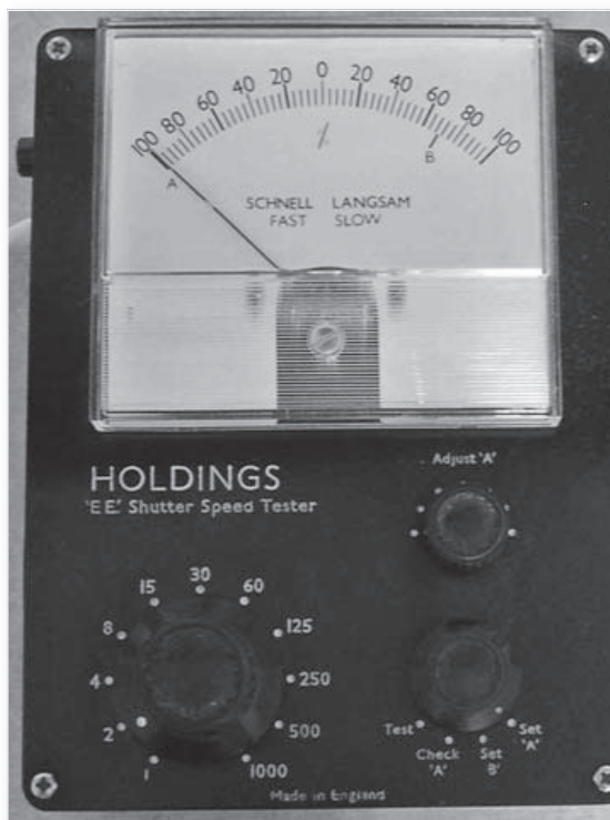
Fig. 3: The production units of the camera shutter tester designed by Harry G3LLL looked rather professional.
